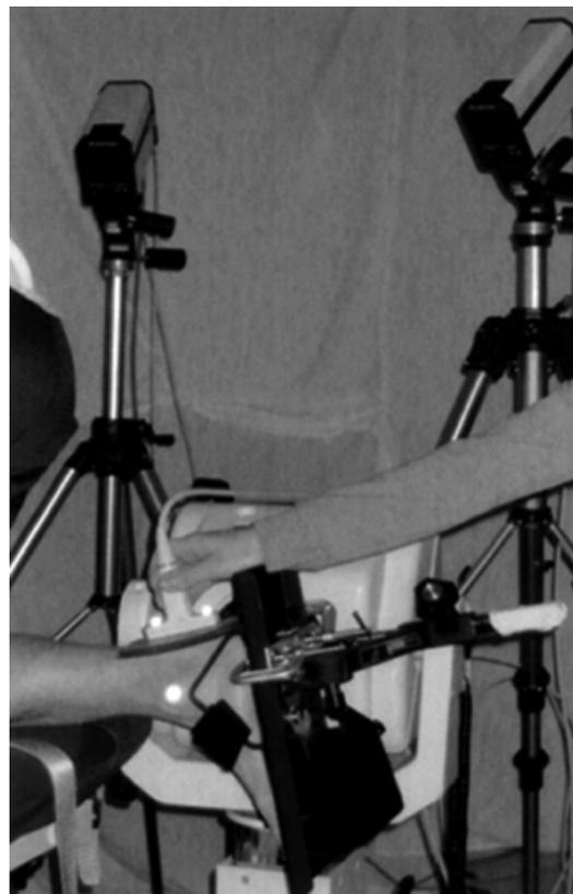
**Figure 1.** Subjects faced the back of the Biodex chair with the foot securely fastened to the foot plate. The ultrasound probe was positioned directly over the Achilles tendon and between the markers over the malleoli. Note the retroreflective markers on the casing of the ultrasound probe and use of gel pad during imaging.
