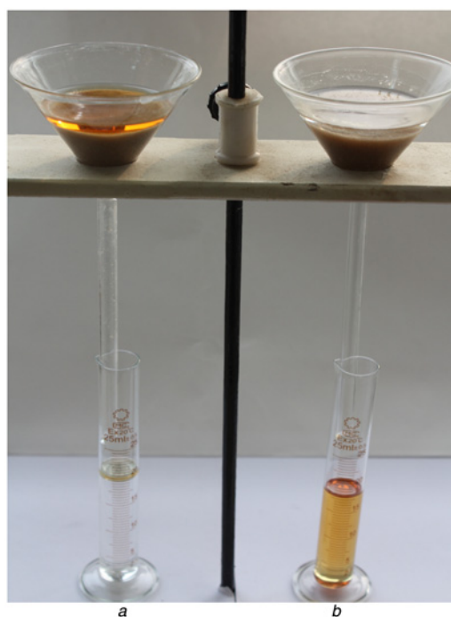
Figure 6 Separation of a mixture of diesel oil and water by unmodified quartz sand (Fig. 6a), and modified quartz sand (Fig. 6b)
