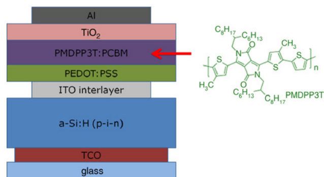
Figure 1 Schematic of a-Si:H photovoltaic and OPV subcells in hybrid tandem solar cell
