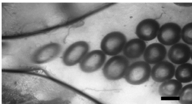
Fig. 7 Droplet generation from the microfluidic chip. Scale bar = 200 \mu\text{m}
