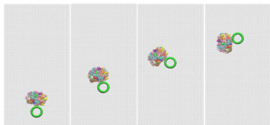
Fig. 4 Top view snapshots of simulation setup CG_6 at the different times. The protein rotates around the tip and the manipulations change from pushing mode to pulling mode (semi-successful pushing)
