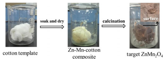
Fig. 1 Graphic formation process of hierarchical porous \text{ZnMn}_2\text{O}_4 , the inserted clearly indicates fibre-like structure of target \text{ZnMn}_2\text{O}_4
