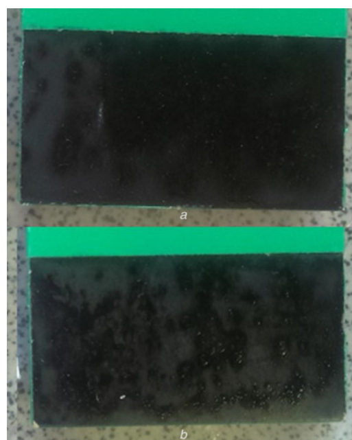
Fig. 2 PPy film electropolymerised on AZ31 Mg alloy a With sodium salicylate pre-treatment b Without sodium salicylate pre-treatment
