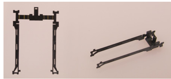
Fig. 5 Photos of the transmission together with the airframe before and after folding
