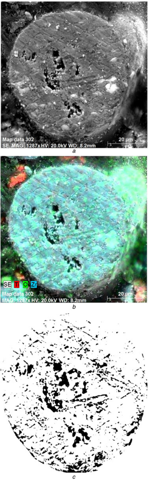
Fig. 3 Morphology of the cross-section mixed YSZ/ \text{TiO}_2 powder before spraying in water is observed a SEM image b Map analysis c Image j analysis of YSZ/ \text{TiO}_2 mixture powders before spraying in water
