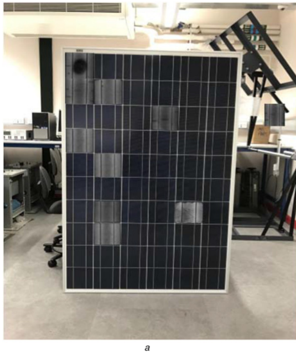
Fig. 6 EL images of cracked solar cells combined with the real images of the examined PV modules
