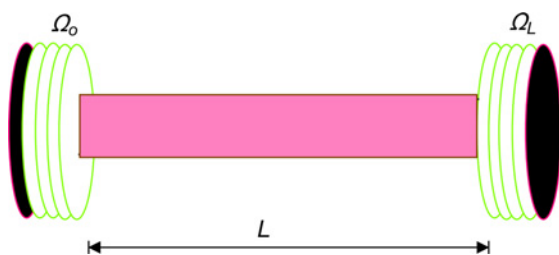
Fig. 1 Nanorod with torsional springs at both ends
