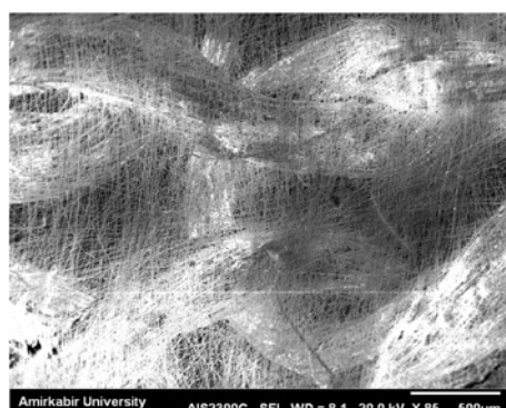
Fig. 3 SEM image of P3HB-Chitosan-MWNT/Silk hybrid nano-micro scaffold
