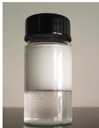
Fig. 6 Distribution of magnesium hydroxide in the mixed solution of water and toluene
