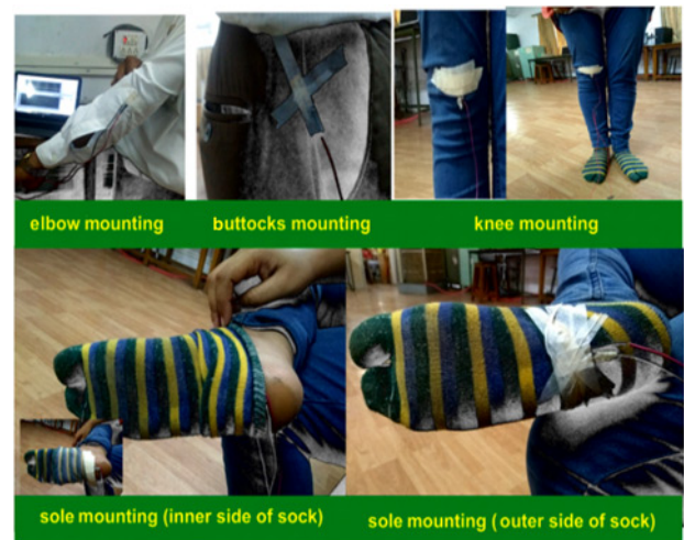
Fig. 12 EHD mounting on energy hot spots
