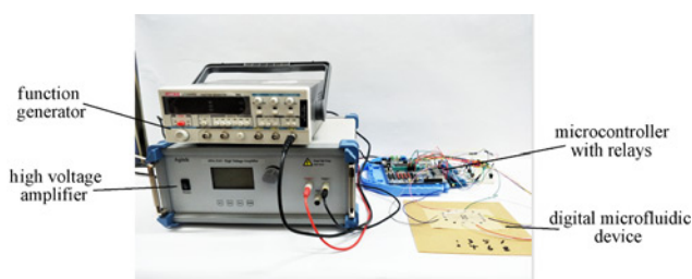
Fig. 4 System setup for the testing of film-based DMF
