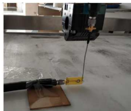
Fig. 8 Homemade magnetic near field probe
