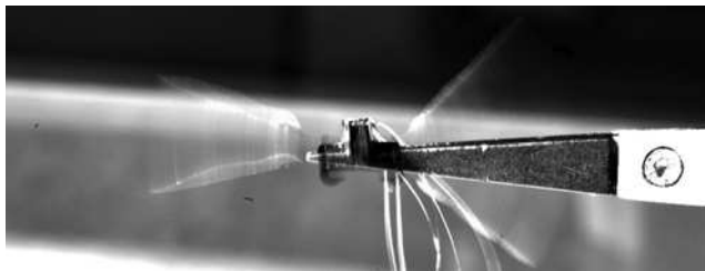
Fig. 3 Asymmetrical flapping of the two wings of the designed robot
