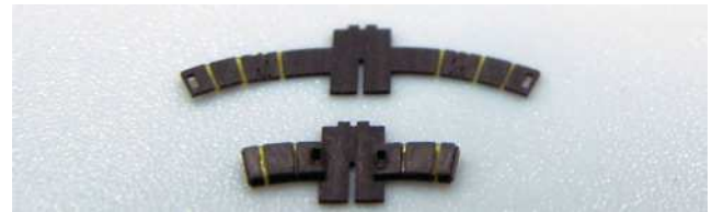
Fig. 5 Photograph of the transmission before and after folding
