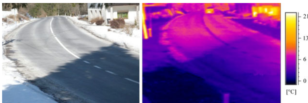
Figure 1. Thermal image showing a variation of the surface temperature on the road section near Ravbarkomanda in the southwestern part of Slovenia. (Source: Articon d.o.o.). This figure is available in colour online at wileyonlinelibrary.com/journal/met
