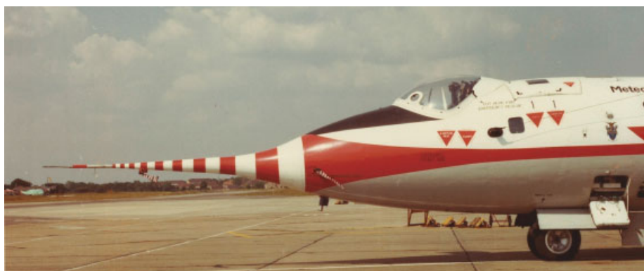
Figure 1. The nose boom installed on the Canberra aircraft used by MRF.
