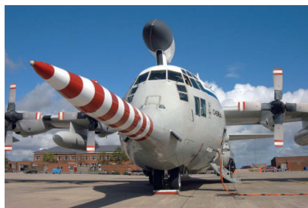
Figure 2. The nose boom installed on the C-130 Hercules aircraft used by MRF. The aircraft radar has been relocated above the cockpit to accommodate the nose boom's installation.
