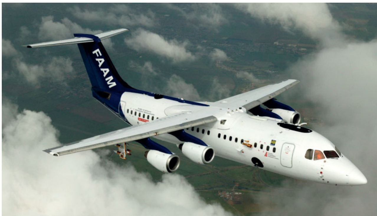
Figure 6. The FAAM research aircraft. Some of the probes which can be seen in this image include cloud physics probes (under the wing), and core thermodynamic probes (below the cockpit window).
