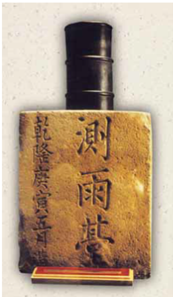
Figure 5. Chukwooki, an old Korean rain gauge used in the Choson Dynasty (the above Chukwooki was known to be made around 1770 in Korea).
