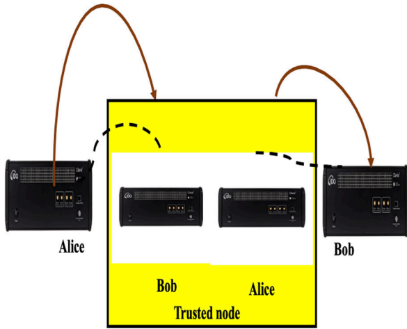
Fig. 3 QKD link via trusted nodes
