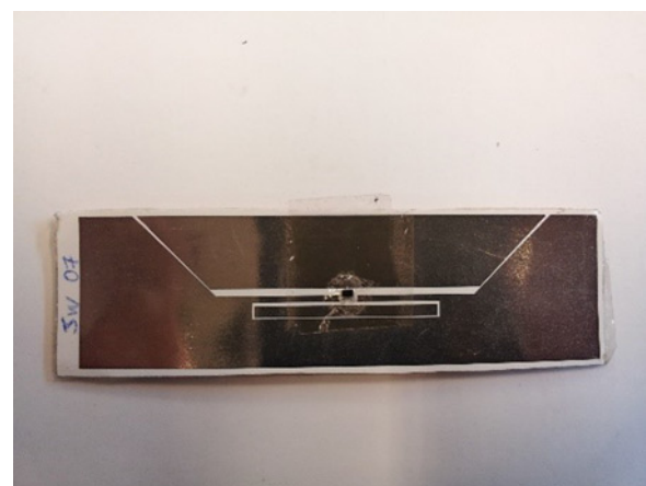
Fig. 3 Inkjet printed tag using conductive ink
