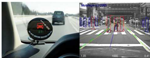
Fig. 3 ADAS system and pedestrian detection diagram
