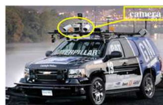
Fig. 9 CMU BOSS intelligent car camera layout
