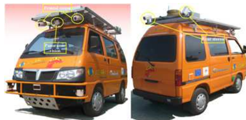
Fig. 7 Porter intelligent car camera layout
