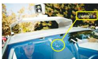
Fig. 4 Google autonomous car camera layout
