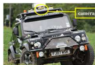
Fig. 8 Bowler Wildcat intelligent car camera layout
