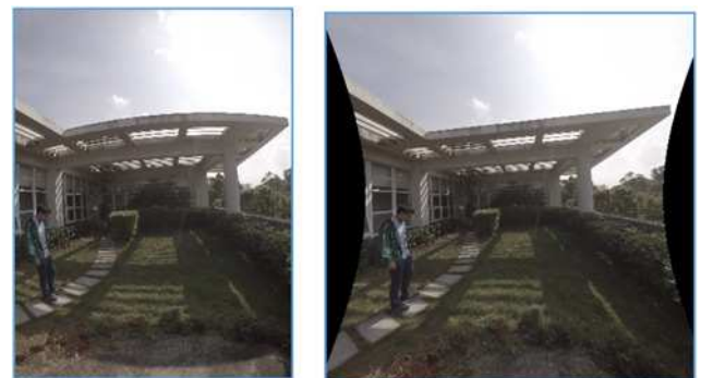
Fig. 5 Left image is one frame of a video captured by a GoPro camera. The fish-eye influence is obvious that the straight lines of buildings are curving. Applying the OCamCalib Toolbox, we get the right image out of fish-eye influence. Apparently, all the straight lines are put back to normal, the scene is nature and confirms the reality
