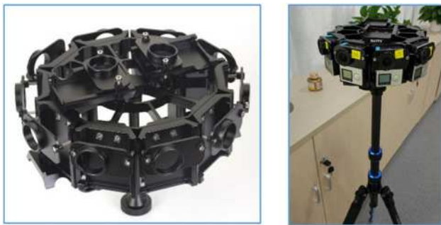
Fig. 2 Our camera rig. There are ten camera positions on the side ring. To get the top and bottom of a panorama, we can choose to place another four cameras
