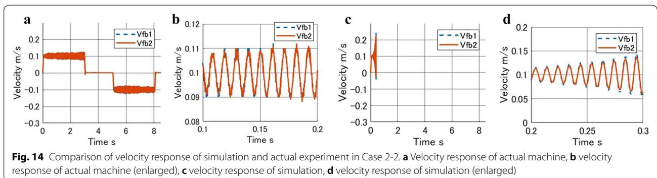
**Fig. 14** Comparison of velocity response of simulation and actual experiment in Case 2-2. **a** Velocity response of actual machine, **b** velocity response of actual machine (enlarged), **c** velocity response of simulation, **d** velocity response of simulation (enlarged)
