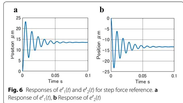
**Fig. 6** Responses of  $e'_1(t)$  and  $e'_2(t)$  for step force reference. **a** Response of  $e'_1(t)$ , **b** Response of  $e'_2(t)$
