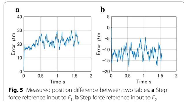
**Fig. 5** Measured position difference between two tables. **a** Step force reference input to  $F_1$ , **b** Step force reference input to  $F_2$
