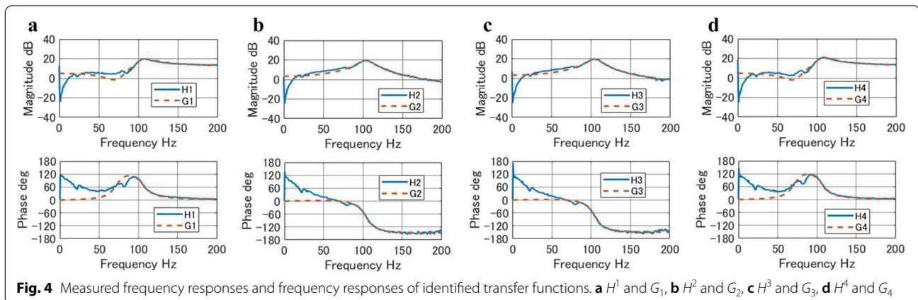
**Fig. 4** Measured frequency responses and frequency responses of identified transfer functions. **a**  $H^1$  and  $G_1$ , **b**  $H^2$  and  $G_2$ , **c**  $H^3$  and  $G_3$ , **d**  $H^4$  and  $G_4$
