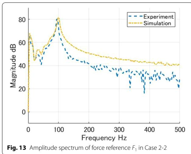
**Fig. 13** Amplitude spectrum of force reference  $F_1$  in Case 2-2
