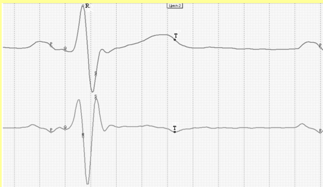
Figure 7. The R point is identified on the ECG as the top of the QRS complex in a similar way as described in other reference literature. This is the only point which is found by criteria other than those used for the phase identification procedure according to the derivative extrema.
