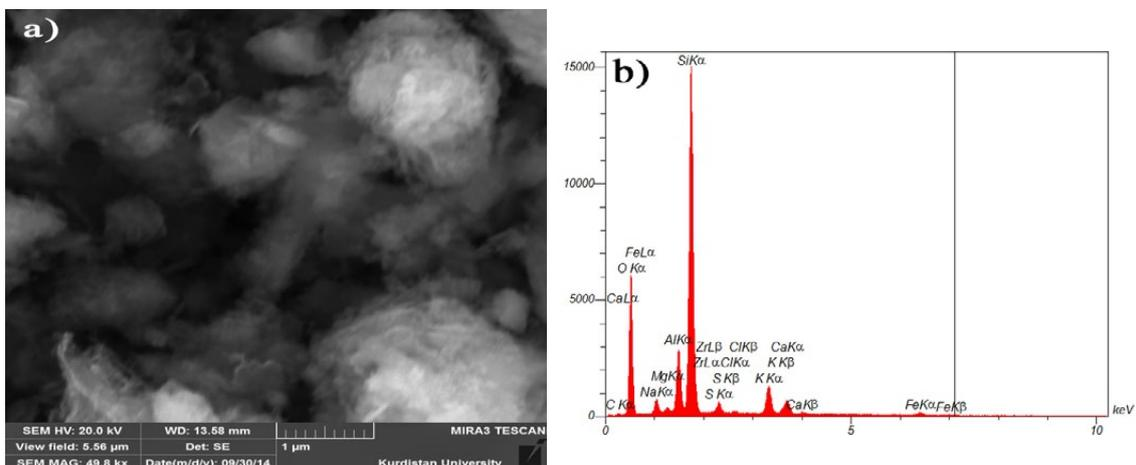
Fig. 2. Scanning electron microscopy (SEM) image (a) and EDX analysis (b) of nanozeolite
