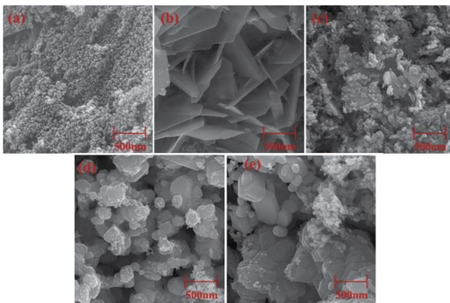
Fig. 5. FE-SEM images of different CdO-ZnO samples
