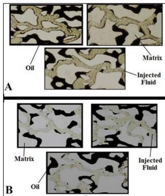
Fig. 13. Pore scale photos of different parts of micromodel glass: A) Ethanol injection and B) Ethanol-silica injection
