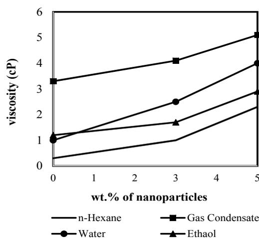
Fig. 5. Change in viscosity versus wt.% of silica nanoparticle in different base fluids
