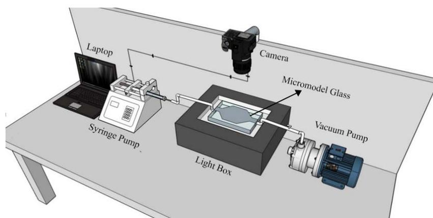
Fig. 2. Schematic of the micromodel Setup
