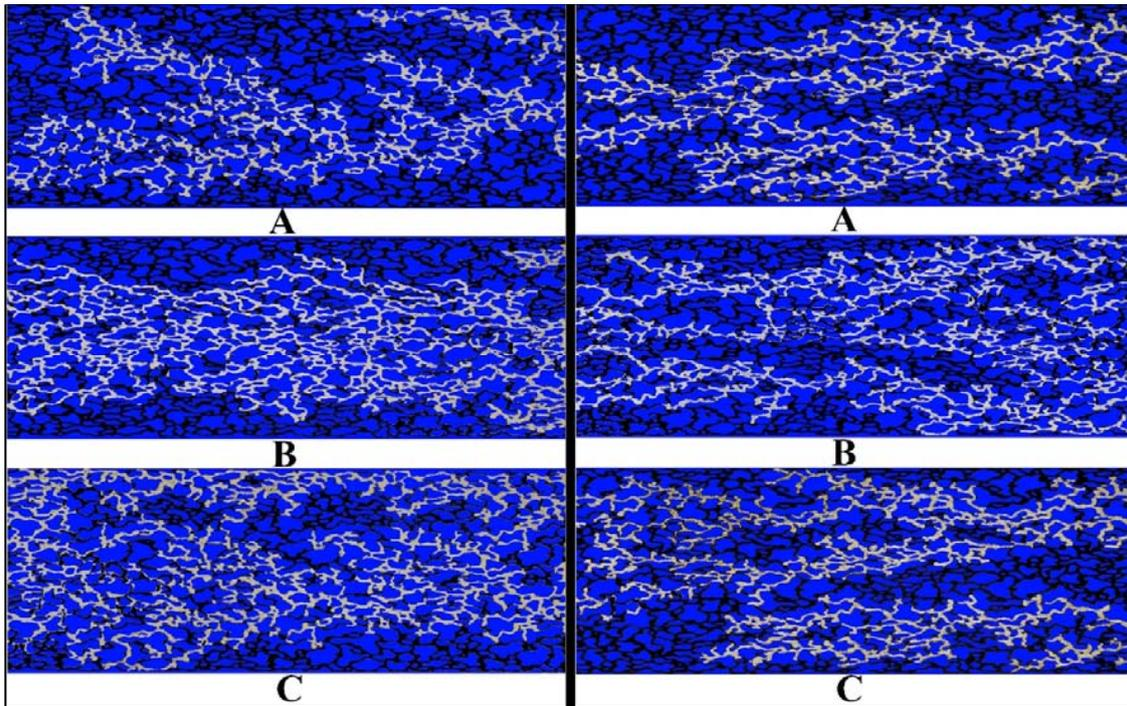
Fig. 6. Macroscopic photos of ultimate recovery for water (left) and Ethanol (Right) base fluid: A) 0 wt.%, B) 3 wt.% and C) 5 wt.% of silica nanoparticles
