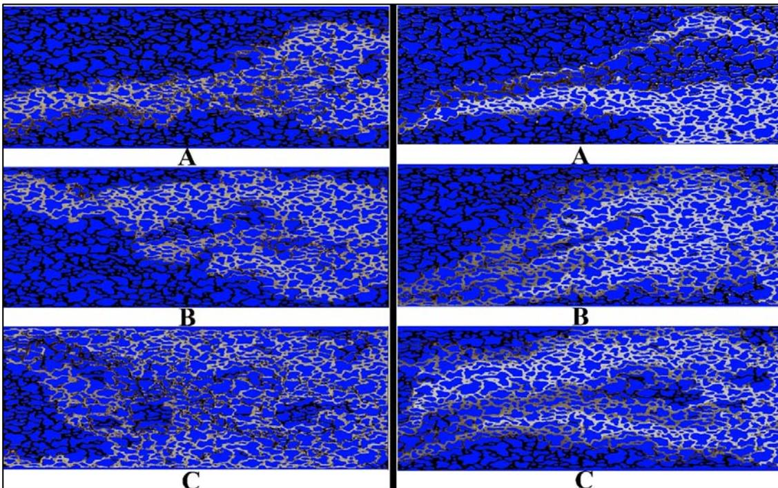
Fig. 7. Macroscopic photos of ultimate recovery for n-hexane (left) and gas condensate (Right) base fluid: A) 0 wt.%, B) 3 wt.% and C) 5 wt.% of silica nanoparticles
