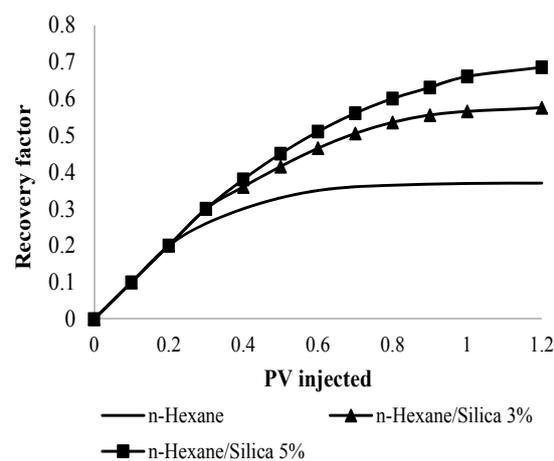
Fig. 10. Oil recovery factor for n-Hexane base nanofluids
