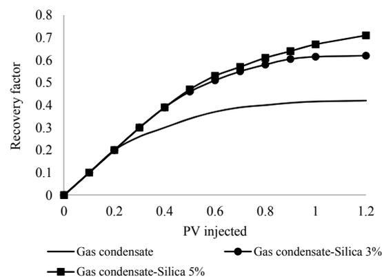
Fig. 11. Oil recovery factor for gas condensate base nanofluids
