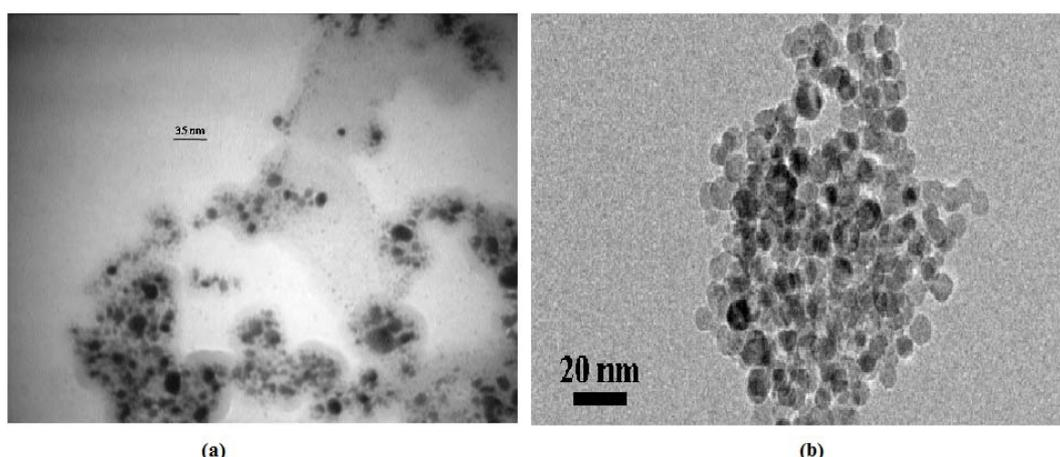
Fig. 1. (a) TEM and (b) SEM image of silica nanoparticles.
