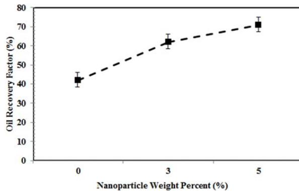
Fig. 16. Effect of nanoparticle's weight percent on the oil recovery
