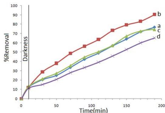
Fig. 8: Photocatalytic removal of 2,4-DCP over a) MWCNTs/ Co-TiO<sub>2</sub> (3.03), b) MWCNTs/ Co-TiO<sub>2</sub> (3.13), c) MWCNTs/ Co-TiO<sub>2</sub> (3.52) and d) MWCNTs/ Co-TiO<sub>2</sub> (4.14) (2,4-DCP Conc. 40 mg/L, 10 mg catalyst, 100 mL 2,4-DCP, visible light, irradiation time: 180 min and H<sub>2</sub>O<sub>2</sub> conc. 0.01M).
