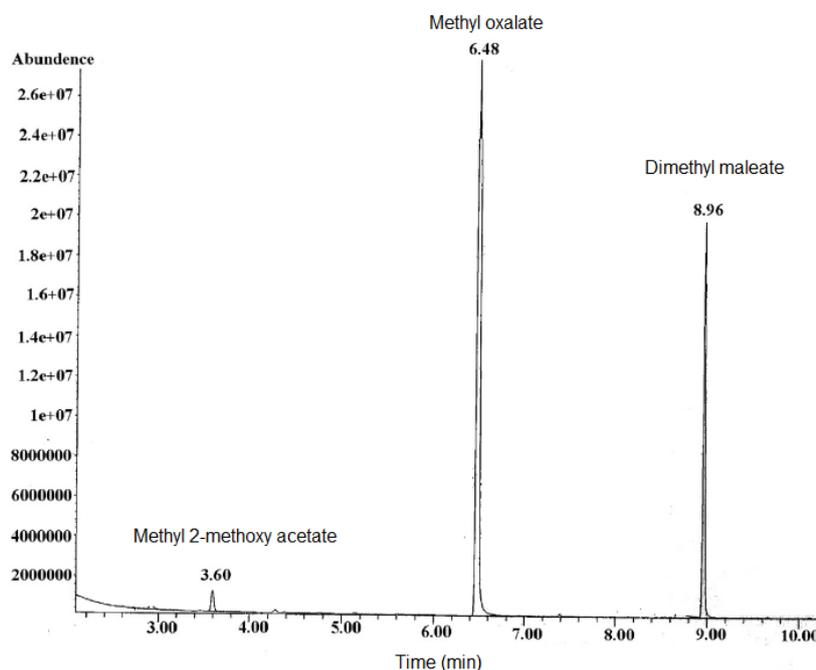
Fig. 10: GC chromatogram of the final products of the photocatalytic degradation of 2,4-DCP by MWCNTs/Co-TiO<sub>2</sub> (3.13).
