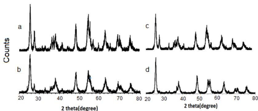
Fig. 2: The XRD patterns of a) MWCNTs/ Co-TiO<sub>2</sub> (3.03), b) MWCNTs/ Co-TiO<sub>2</sub> (3.13), c) MWCNTs/ Co-TiO<sub>2</sub> (3.52) and d) MWCNTs/ Co-TiO<sub>2</sub> (4.14)
