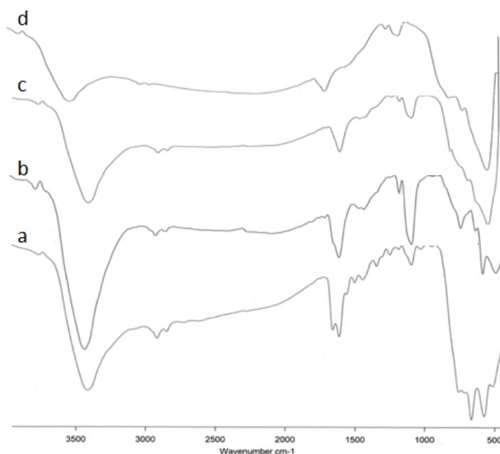
Fig. 6: FTIR spectra of a) MWCNTs/ Co-TiO<sub>2</sub> (3.03), b) MWCNTs/ Co-TiO<sub>2</sub> (3.13), c) MWCNTs/ Co-TiO<sub>2</sub> (3.52) and d) MWCNTs/ Co-TiO<sub>2</sub> (4.14).
