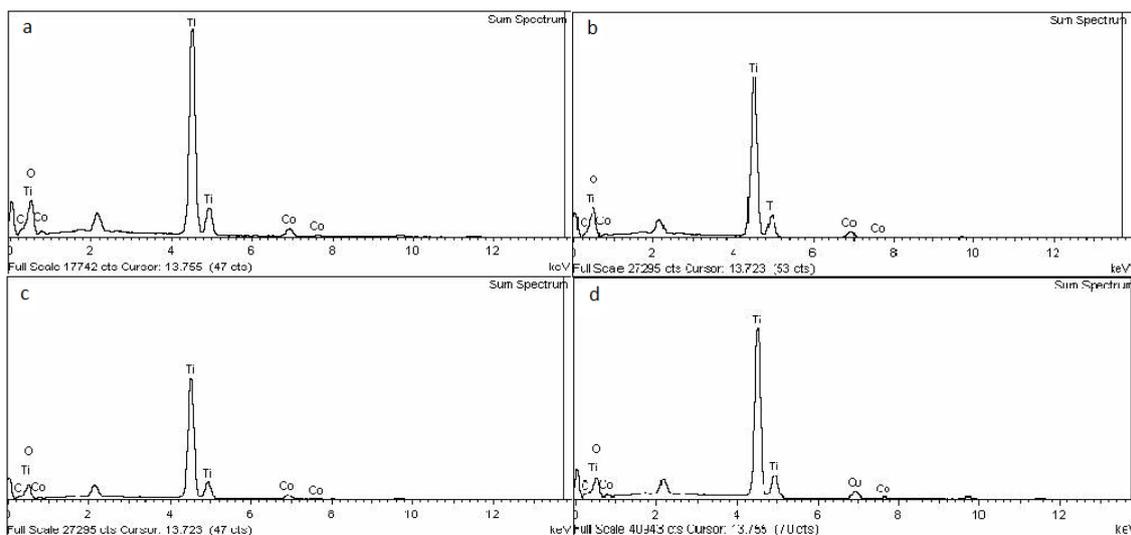
Fig. 4: EDX patterns of a) MWCNTs/ Co-TiO<sub>2</sub> (3.03), b) MWCNTs/ Co-TiO<sub>2</sub> (3.13), c) MWCNTs/ Co-TiO<sub>2</sub> (3.52) and d) MWCNTs/ Co-TiO<sub>2</sub> (4.14).
