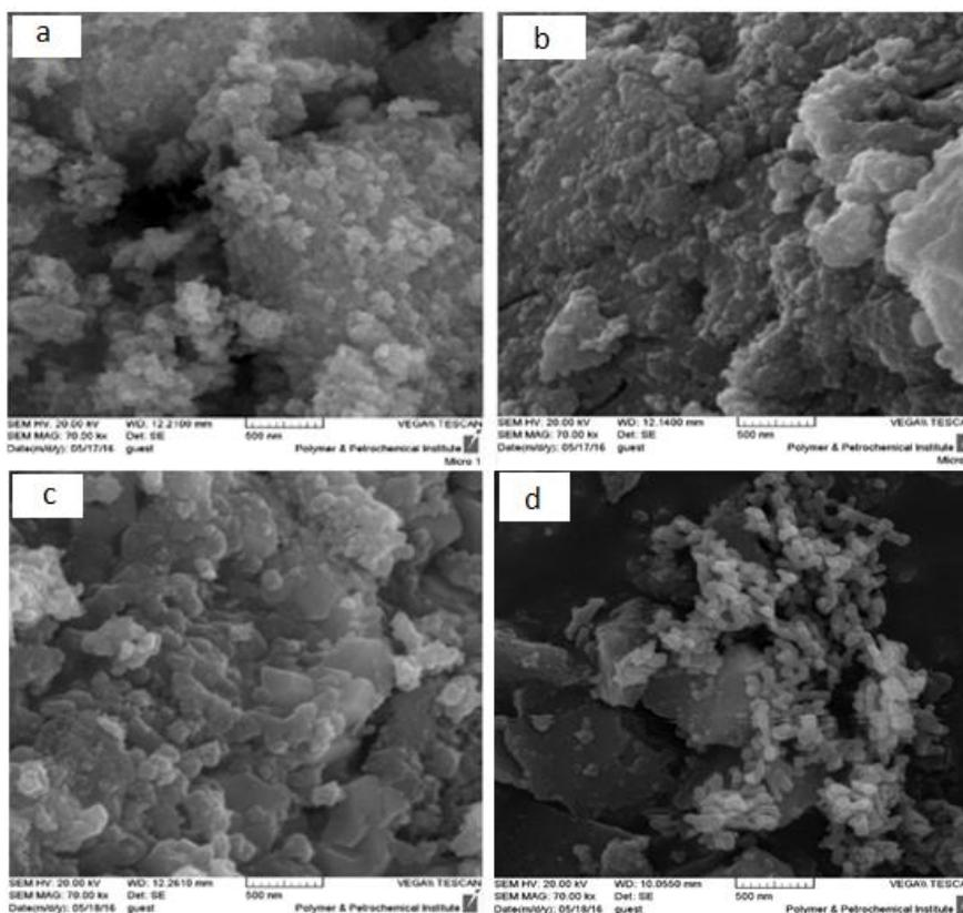
Fig. 3: SEM micrographs of a) MWCNTs/ Co-TiO<sub>2</sub> (3.03), b) MWCNTs/ Co-TiO<sub>2</sub> (3.13), c) MWCNTs/ Co-TiO<sub>2</sub> (3.52) and d) MWCNTs/ Co-TiO<sub>2</sub> (4.14)
