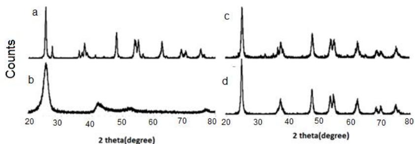
Fig. 1: The XRD patterns of a) TiO<sub>2</sub>, b) MWCNTs, c) MWCNTs/TiO<sub>2</sub> and d) Co-TiO<sub>2</sub>
