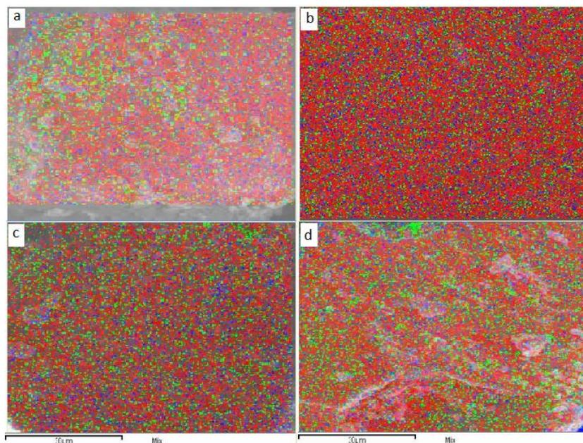
Fig. 5: Elemental mapping images of a) MWCNTs/ Co-TiO<sub>2</sub> (3.03), b) MWCNTs/ Co-TiO<sub>2</sub> (3.13), c) MWCNTs/ Co-TiO<sub>2</sub> (3.52) and d) MWCNTs/ Co-TiO<sub>2</sub> (4.14).
