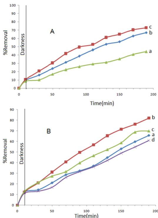
Fig. 7: Photocatalytic degradation of 2,4-DCP over A: (a) TiO<sub>2</sub>, b) Co-TiO<sub>2</sub> and c) MWCNTs/TiO<sub>2</sub>, B: a) MWCNTs/ Co-TiO<sub>2</sub> (3.03), b) MWCNTs/ Co-TiO<sub>2</sub> (3.13), c) MWCNTs/ Co-TiO<sub>2</sub> (3.52) and d) MWCNTs/ Co-TiO<sub>2</sub> (4.14) (2,4-DCP Conc. 40 mg/L, 10 mg catalyst, 100 mL 2,4-DCP, visible light, irradiation time: 180 min).
