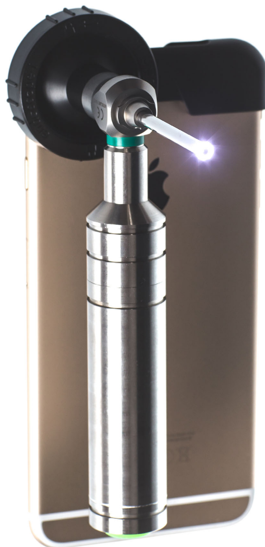
FIGURE 1 Light wand fitted with adapter and endoscope to iOS device
