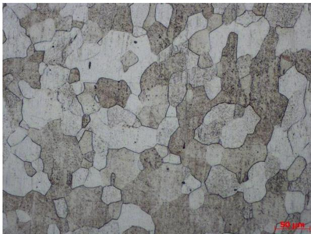
Fig. 2. Optical micrograph of the initial steel.
