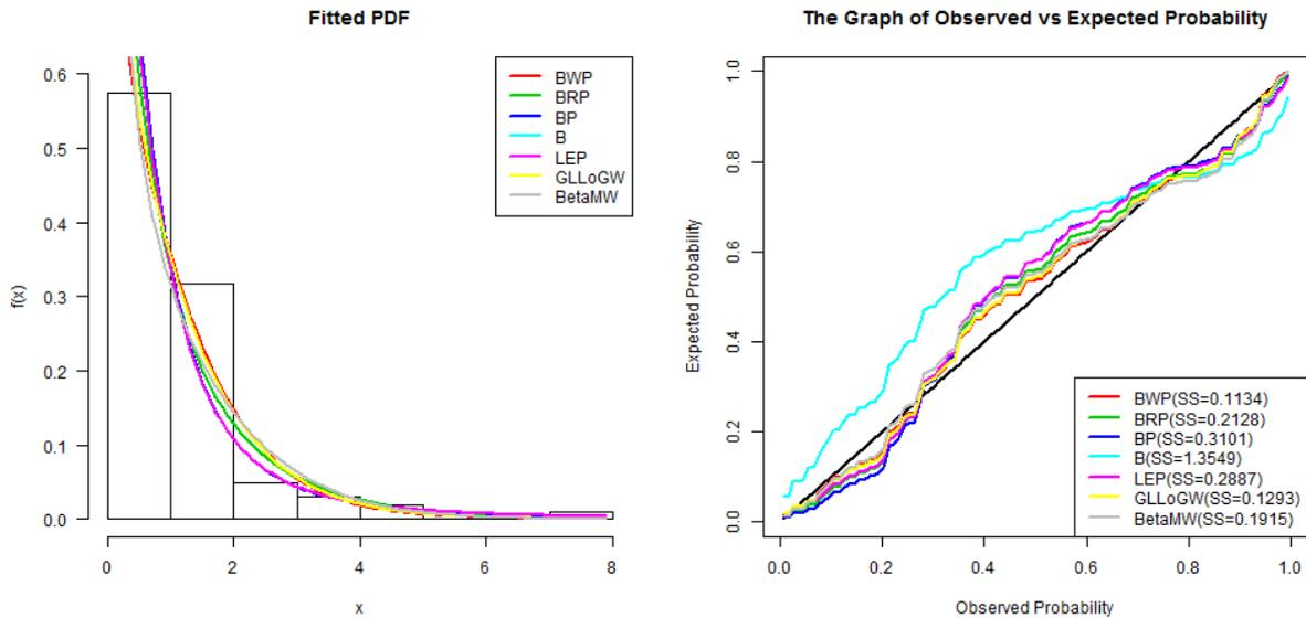
Figure 3: Fitted Densities and Probability Plots for Time to Failure of kevlar 49/epoxy strands tested at various stress level data
