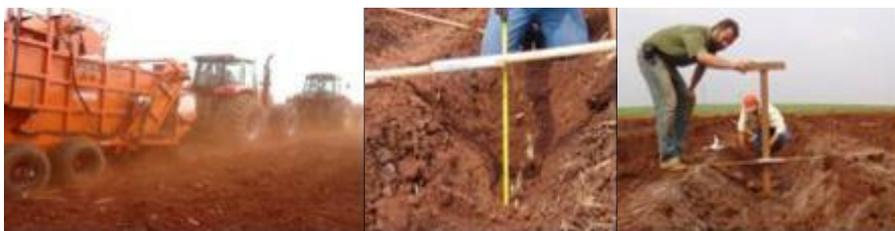
FIGURE 3. Determinations of (A) drawbar force; (B) furrow depth and (C) amount of soil over the billets.
