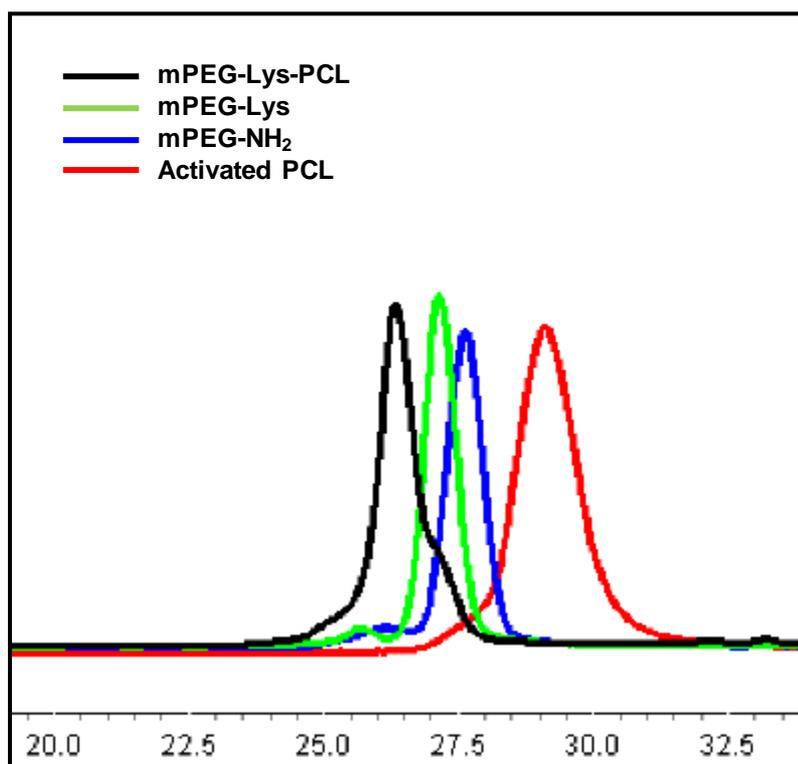
**Figure 5.** GPC traces of PCL, mPEG-NH<sub>2</sub>, mPEG-Lys and mPEG-Lys-PCL using DMF as an eluent.
