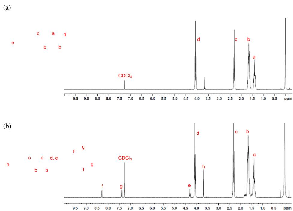
**Figure 3.**  $^1\text{H}$ -NMR spectra of (a) PCL and (b) activated PCL in  $\text{CDCl}_3$ .
