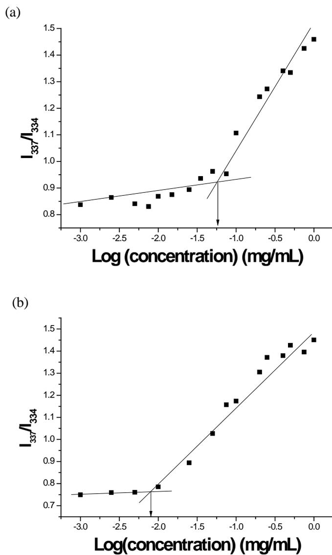
**Figure 8.** The critical micelle concentration (CMC) of (a) non-crosslinked micelle and (b) crosslinked micelle intensity ratio ( $I_{337}/I_{334}$ ) from pyrene excitation spectra as a function of polymer concentration in PBS (pH 7.4).
