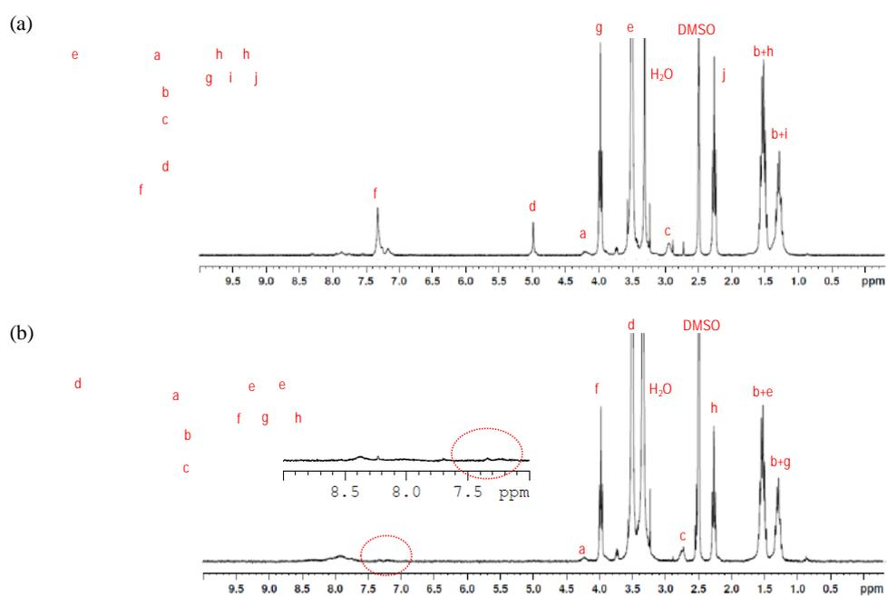
**Figure 4.** <sup>1</sup>H-NMR spectra of mPEG-Lys-PCL (a) before deprotection and (b) after deprotection in DMSO-*d*<sub>6</sub>.
