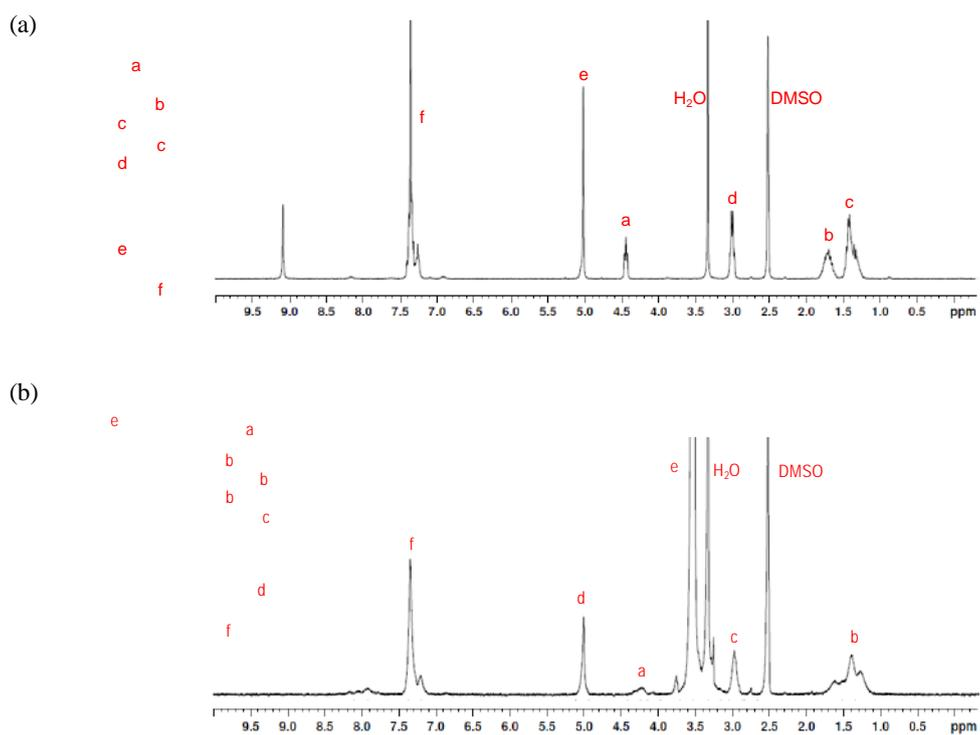
**Figure 2.**  $^1\text{H-NMR}$  spectra of (a) Z-Lysine NCA and (b) mPEG-Lys(Z) in  $\text{DMSO-}d_6$ .
