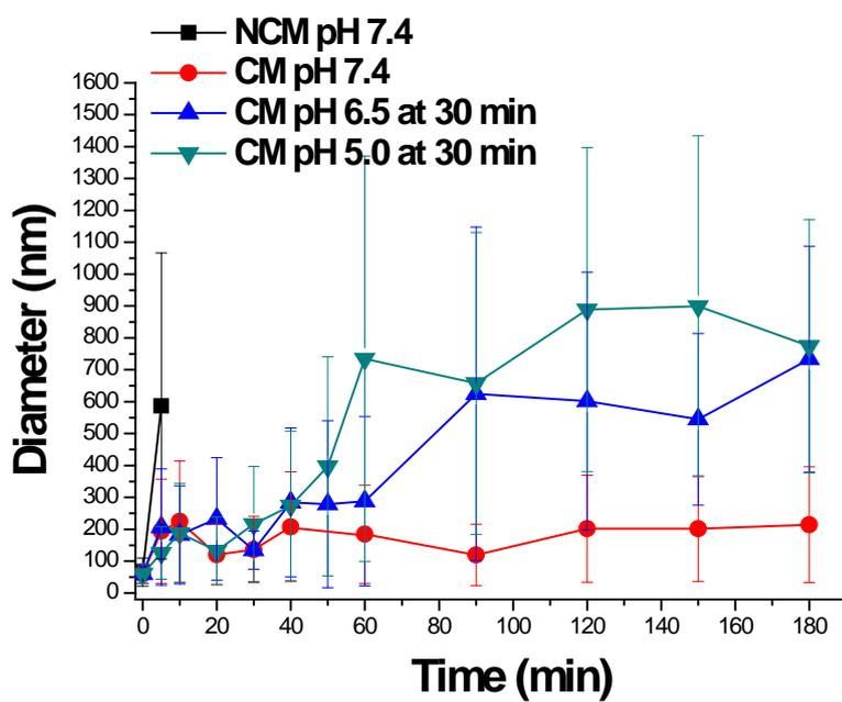
**Figure 9.** The stability in particle size of NCMs and CMs in the presence of 2.5 mg/mL SDS measured by DLS.
