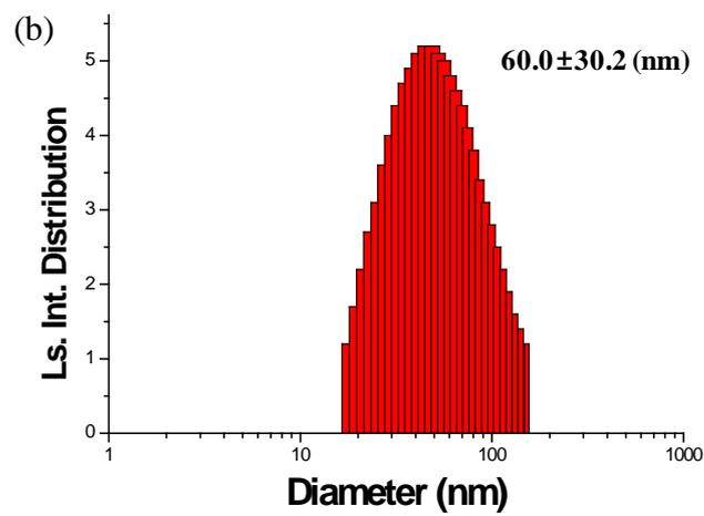
**Figure 6.** Size distribution of (a) non-crosslinked micelles and (b) crosslinked micelles in phosphate buffer at pH 7.4.
