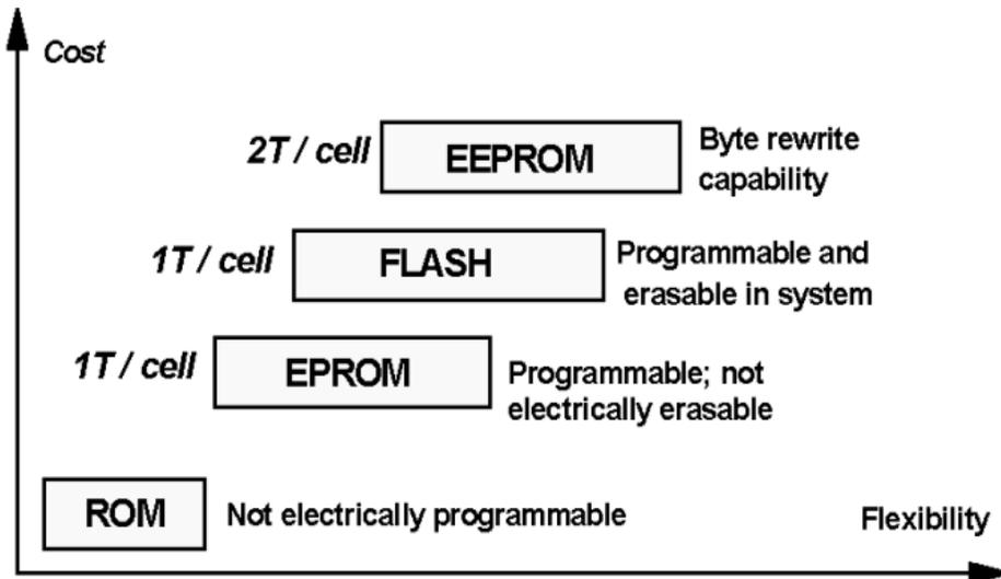
**Figure 2.** Non-volatile memory qualitative compared in terms of flexibility and cost.
