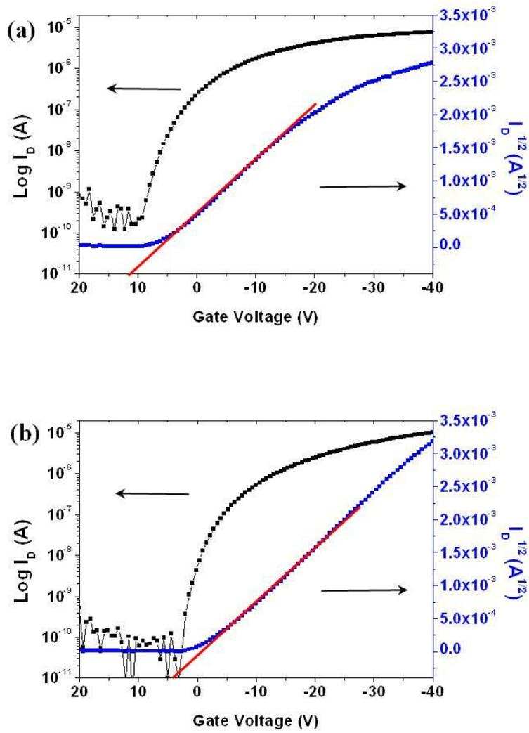
**Figure 8.** Transfer characteristics of OFET-based memory (a) including the myoglobin chargeable layer and (b) excluding the myoglobin chargeable layer at  $V_D = -40$  V.
