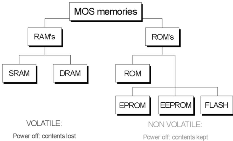
**Figure 1.** The categories of metal-oxide-semiconductor (MOS) memories.
