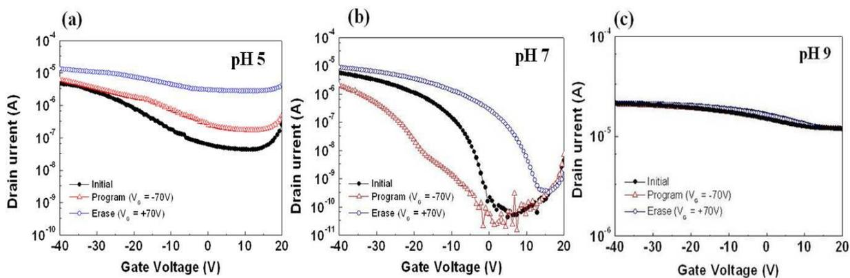
**Figure 11.** Transfer characteristics of OFET-based memory according to the pH of buffer solution using 1mM myoglobin solution after applying programming/erasing operations. The performances have changed with the pH of sodium buffer solution (a) pH 5, (b) pH 7, and (c) pH 9.
