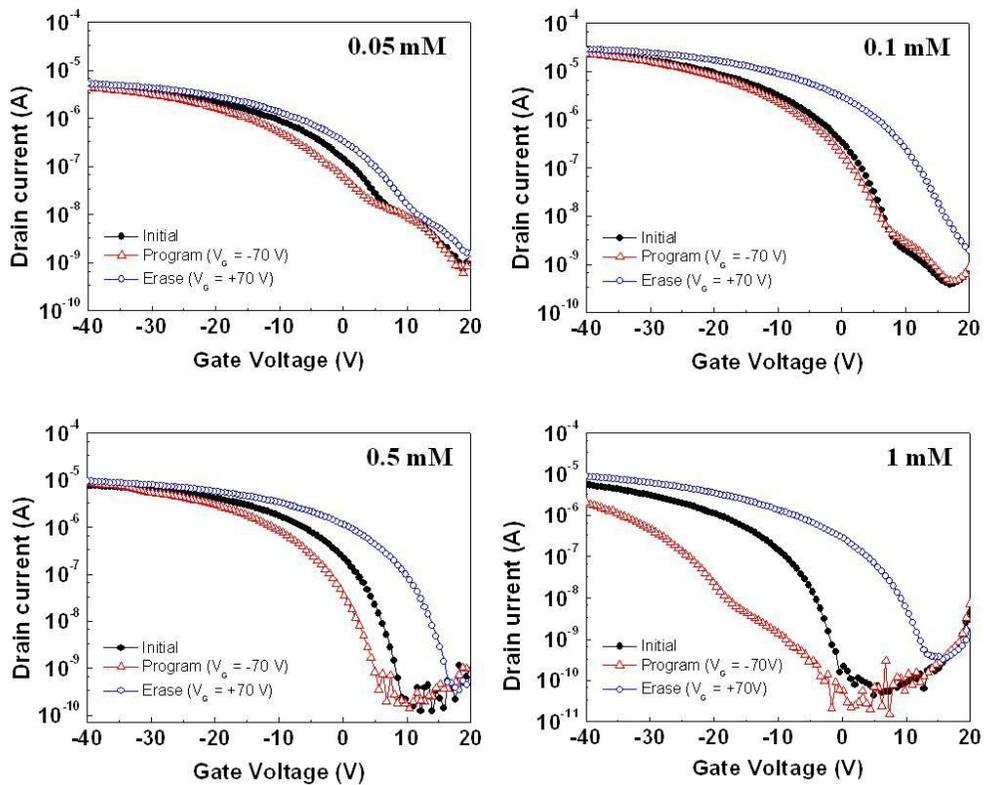
**Figure 10.** Transfer characteristics of OFET-based memory according to the concentration of myoglobin solutions after applying programming/erasing operation.
