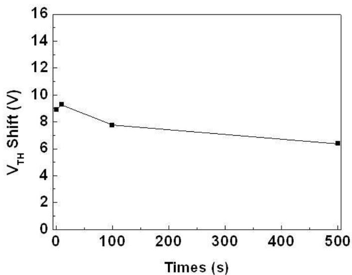
**Figure 13.** Retention characteristics as a function of the retention time for OFET-based memory including the myoglobin chargeable layer prepared using 0.5 mM myoglobin solution. The results were measured in ambient conditions at room temperature.
