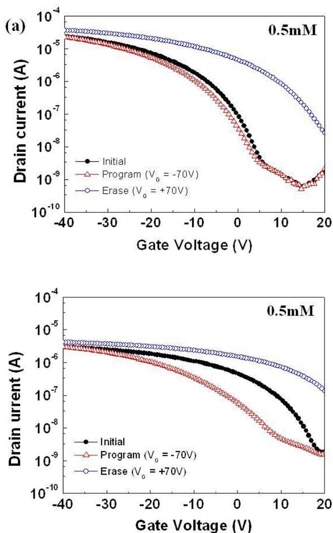
**Figure 14.** Transfer characteristics of OFET-based memory according to other types of redox proteins as a charge trapping element for determining considerable changes of threshold voltage after applying programming/erasing operations: (a) hemoglobin and (b) cytochrome *c*.
