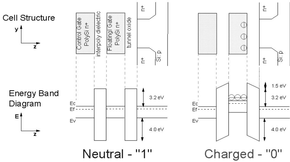
**Figure 4.** Schematic energy band diagram of flash memory with a semiconductor-insulator-metal-insulator-metal sandwich.
