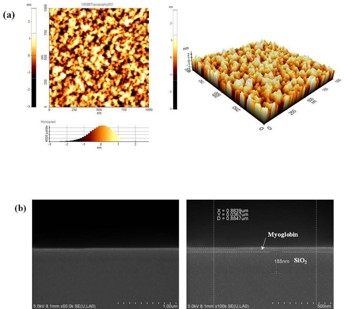
**Figure 7.** (a) AFM images and (b) cross-sectional SEM images of the myoglobin films prepared using 0.5 mM solutions. The myoglobin films were deposited by spin-coating onto  $\text{SiO}_2$  (200 nm) surface thermally grown on Si substrate
