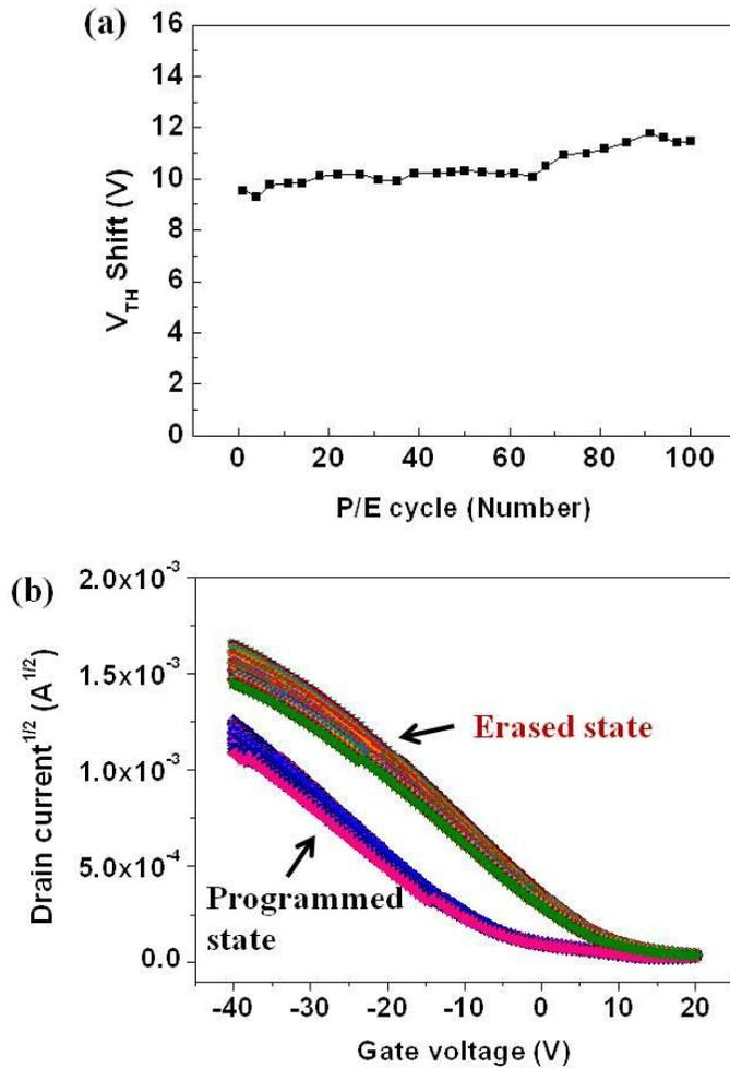
**Figure 12.** Performance of OFET-based memory including the myoglobin chargeable layer prepared using 0.5 mM myoglobin solution. The results were measured in ambient conditions at room temperature: (a) endurance test performed during 100 cycles and (b) transfer characteristics.
