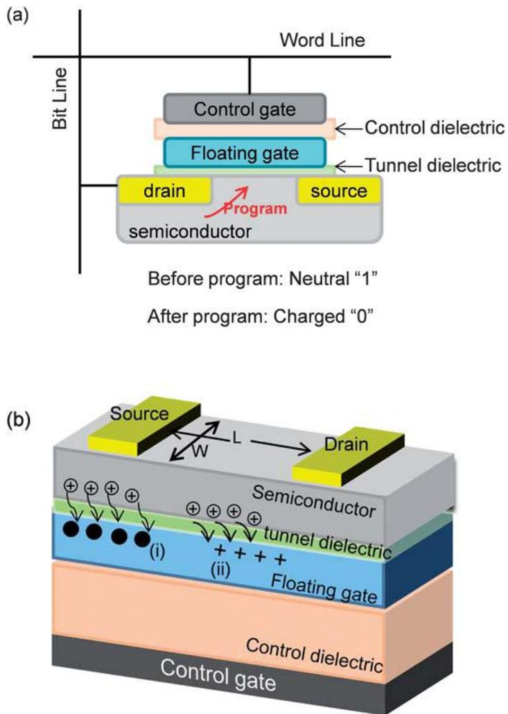
**Figure 3.** Schematic structure of (a) conventional flash memory, (b) charge trapping OFET-based memory device.
