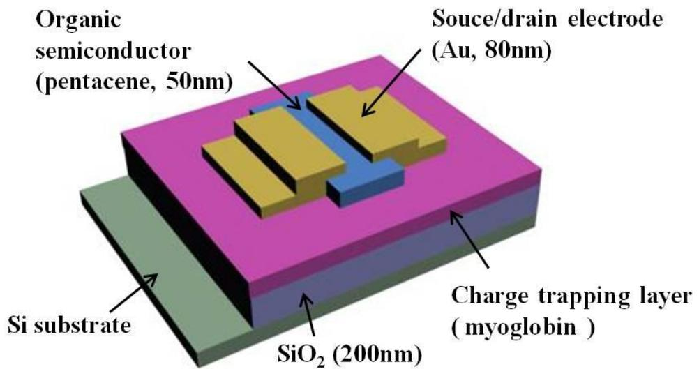
**Figure 5.** Schematic structure of the bottom-gate, top-contact OFET-based memory device including the myoglobin charge trapping layer.
