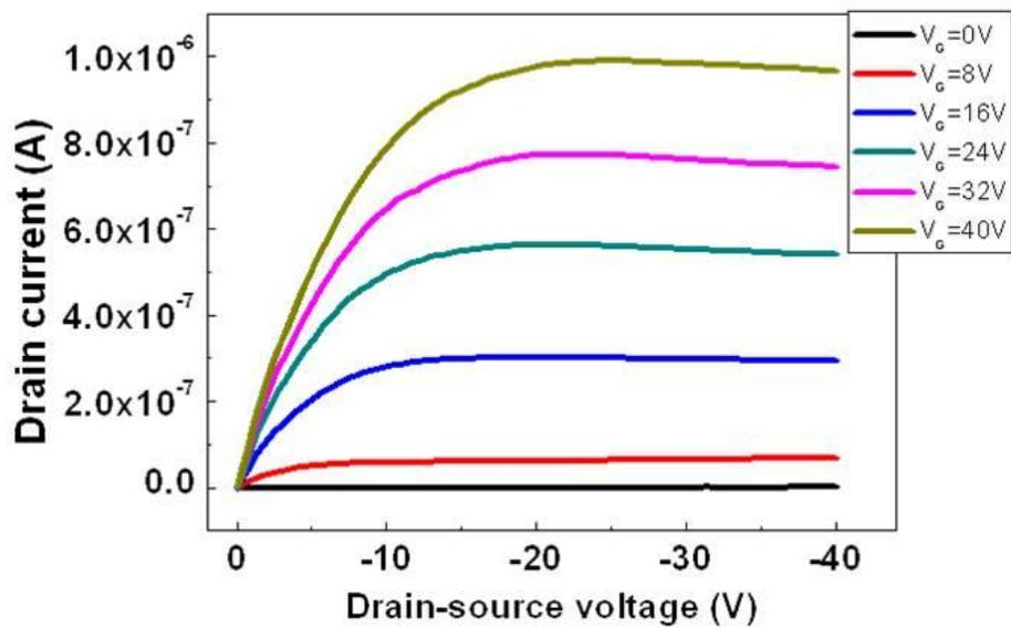
**Figure 9.** Output characteristics of OFET-based memory including the myoglobin chargeable layer prepared using 0.5 mM myoglobin solution. The gate voltage ranges from 0 V to -40 V in 8 V steps.
