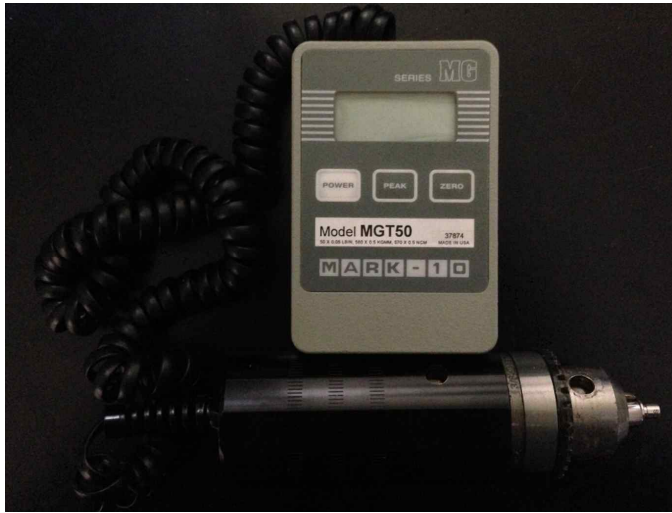
Fig. 3. Digital torque gauge (MGT50)
