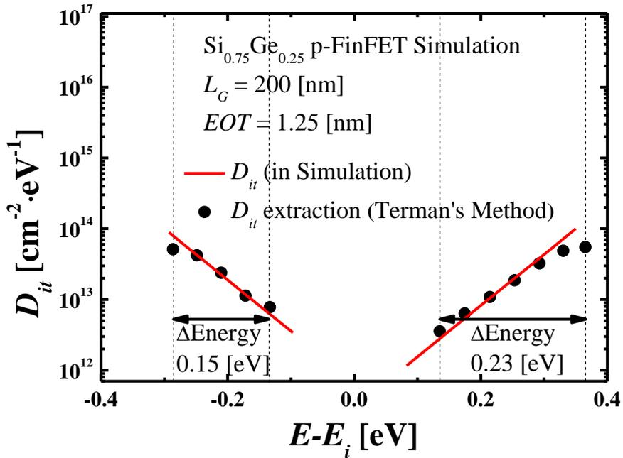
Figure 3. Interface trap density inputted in simulation (red line) and extracted by Terman's method (black dotted line).
