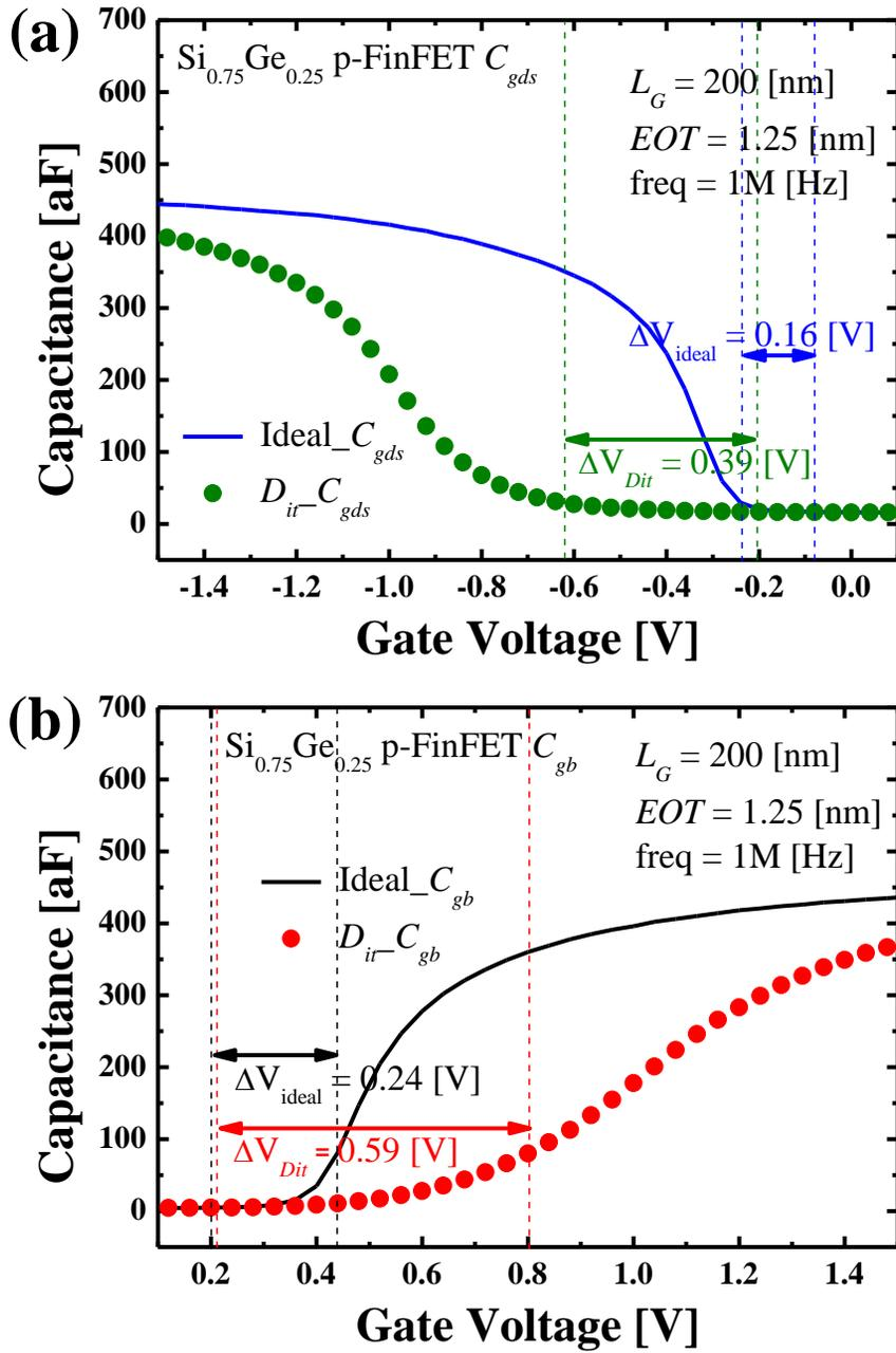
Figure 4. Comparison of voltage difference between ideal and stretch-out C-V curve (a)  $C_{gds}$  and (b)  $C_{gb}$ .
