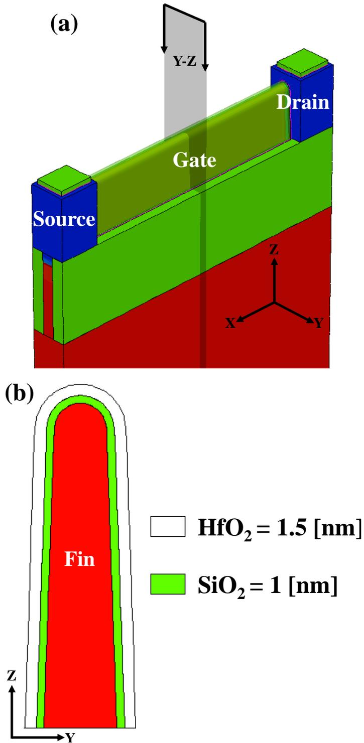
Figure 1. (a) Three-dimensional structure of SiGe p-FinFET.
