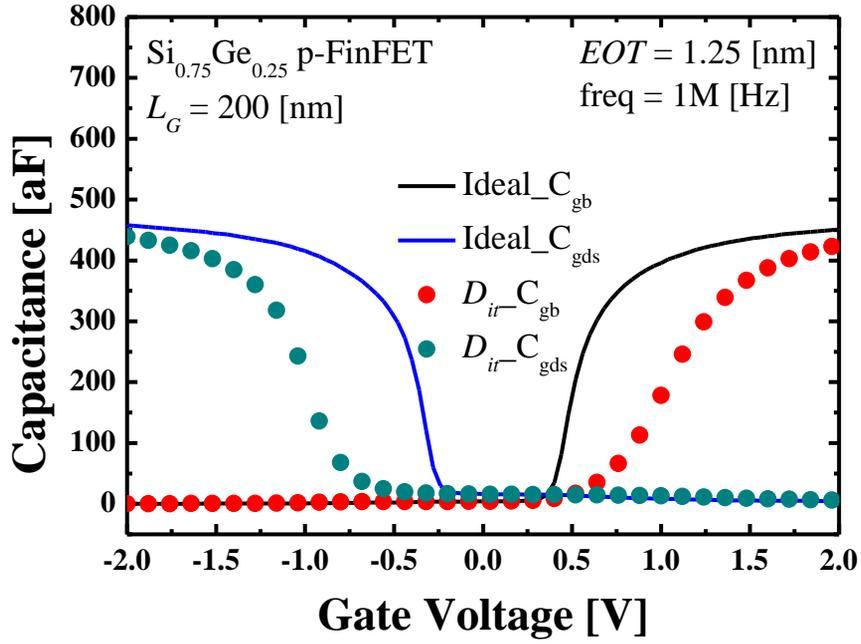
Figure 2. Simulation C-V curve of SiGe p-FinFET.
