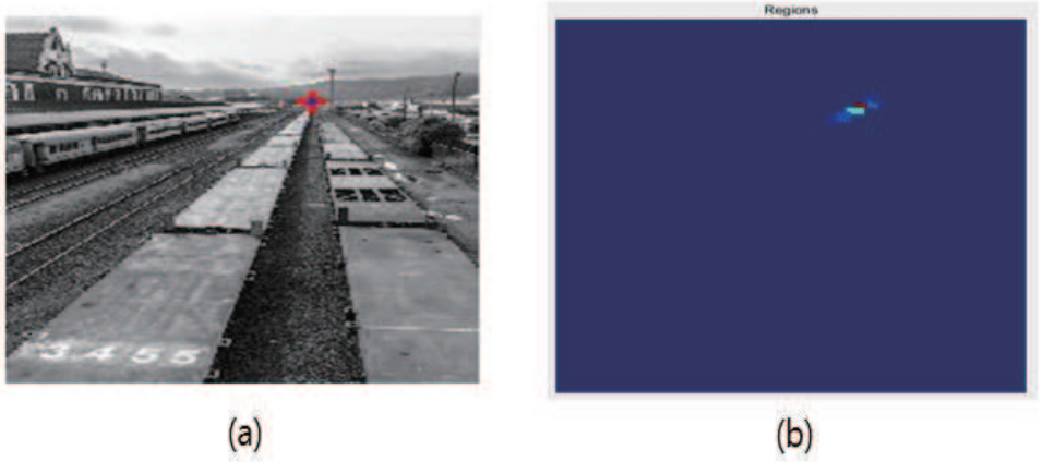
Figure 3.8: Result images of vanishing point and region map on weight sum (a) Original image with vanishing point (b) Region weight sum map (Blue to Red represents low to high value of weight sum.)
