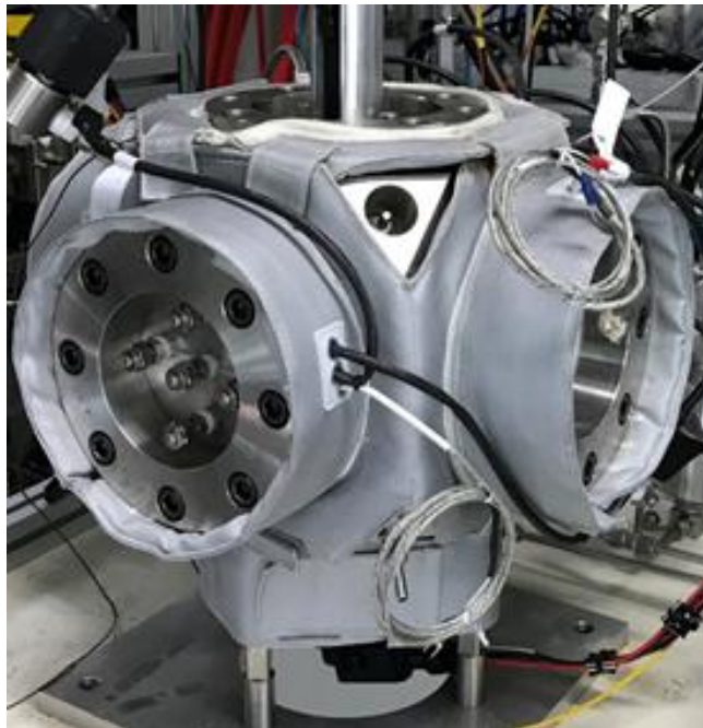
Figure 2.3 Constant volume combustion chamber
