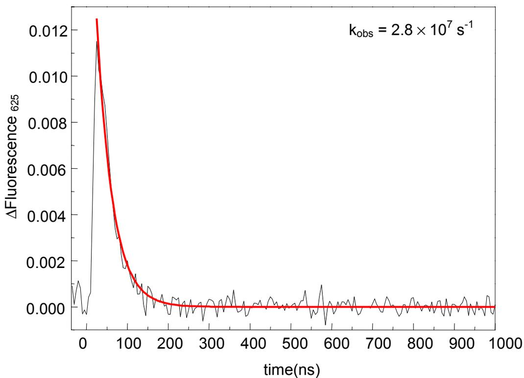
**Figure A.3.** Top: reductive quenching scheme; Q = MeODMA, Fe = heme in DNS(C102)-cyt *c*, Ru = ruthenium center in Ru(bpy)<sub>3</sub>; bottom: kinetic trace for the decay of Ru(bpy)<sub>3</sub><sup>2+</sup>\* triplet excited state in presence of Q.
