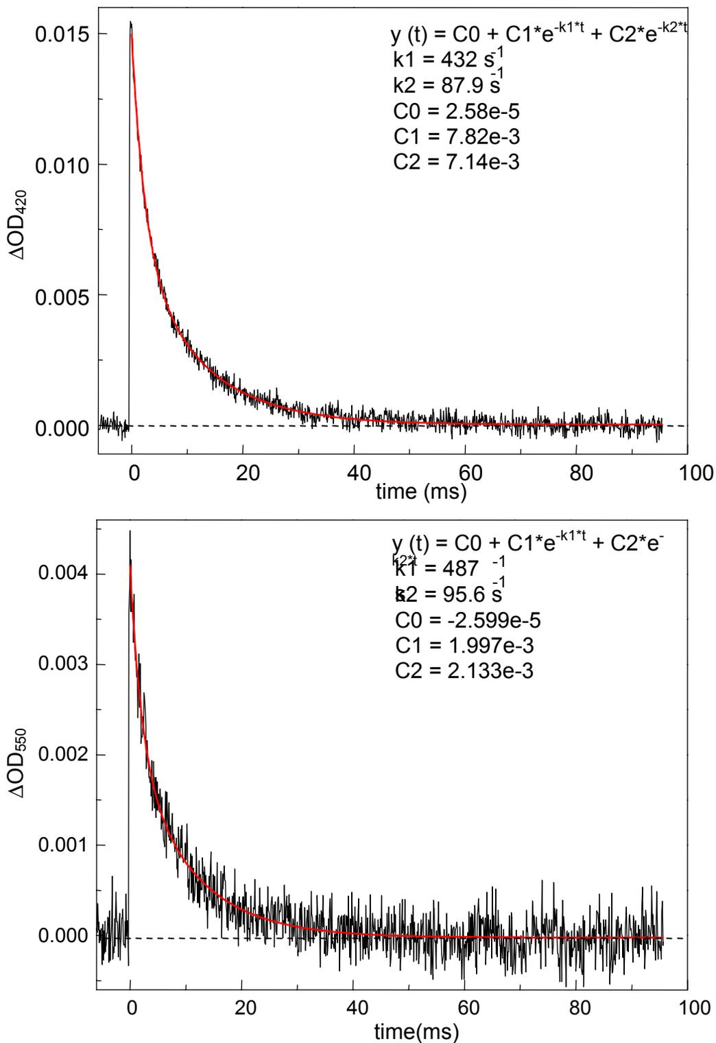
**Figure A.6.** Reoxidation of DNS(C102)-cyt  $c^{III}$ ; top: transient absorption kinetics ( $\lambda_{\text{obs}}=420 \text{ nm}$ ); bottom: transient absorption kinetics ( $\lambda_{\text{obs}}=550 \text{ nm}$ ). Experimental conditions are as in Figure 5.5. The lines are the best fits to a biexponential function.
