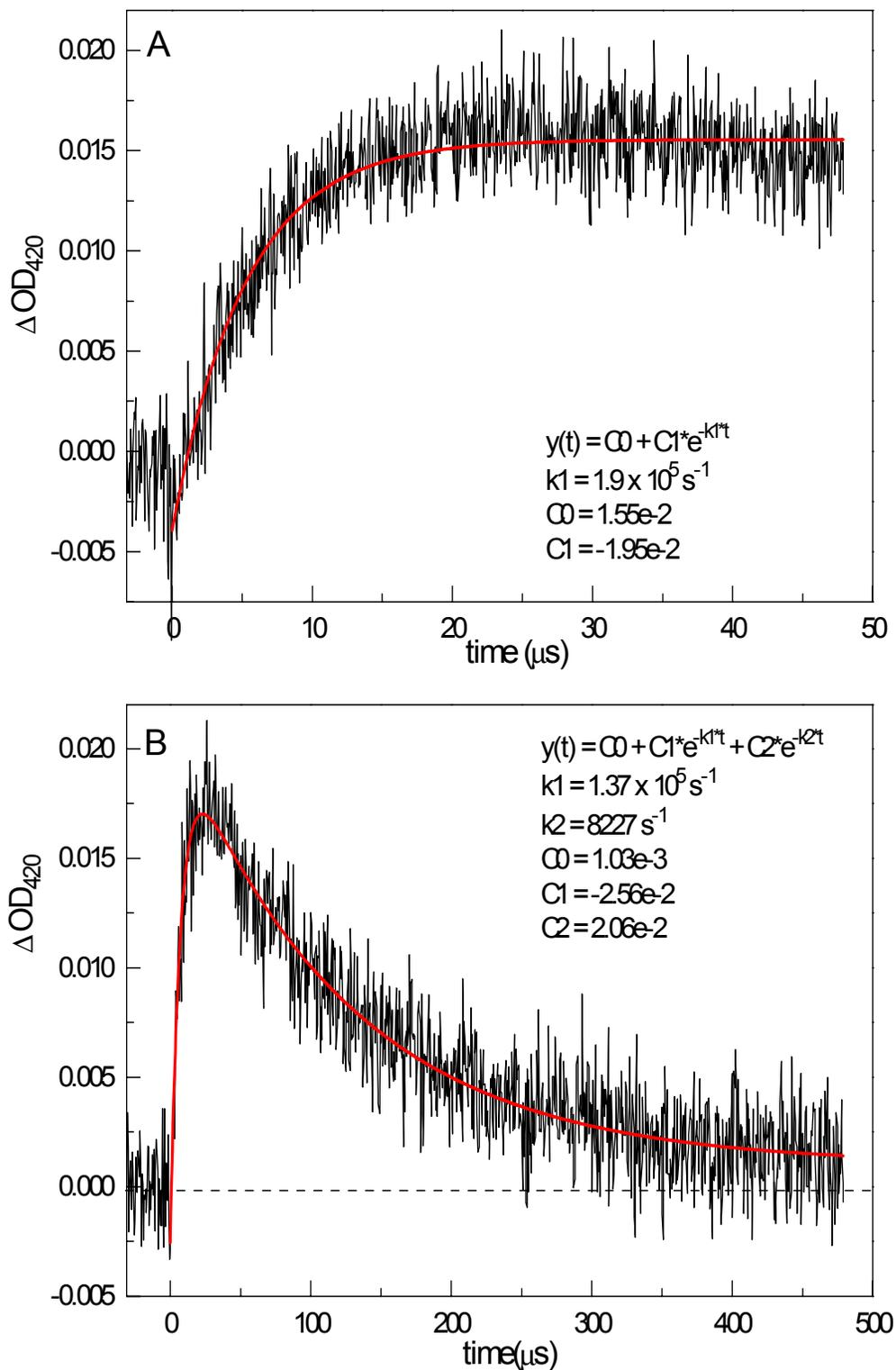
**Figure A.4.** Transient absorption kinetics monitored at 420 nm after excitation ( $\lambda_{ex} = 480$  nm) of 36  $\mu M$  DNS(C102)-cyt c, 10  $\mu M$  Ru(bpy)<sub>3</sub><sup>2+</sup>, 10 mM MeODMA (all in  $\sim 2.8$  M GuHCl, NaPi ( $\mu = 0.1$ , pH 7, 20°C)). The lines are the best fits to single exponential (top) and biexponential (bottom) functions.
