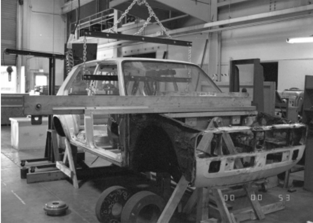
Figure 5.1: Testing setup of body-in-white.
