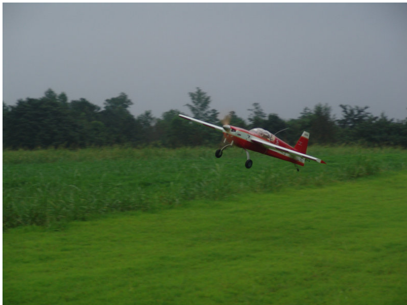
Figure 4: The GTEdge Aircraft with a high (greater than 1) thrust-to-weight ratio
