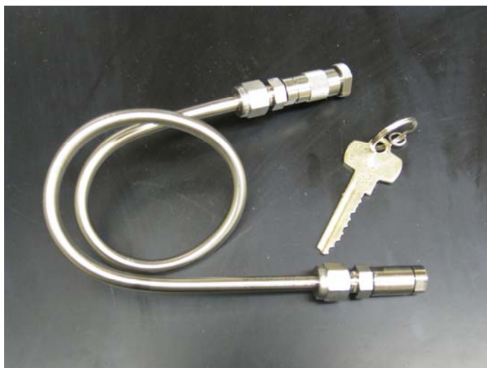
Figure 2-29: Photograph of the coiled continuous flow reactor
