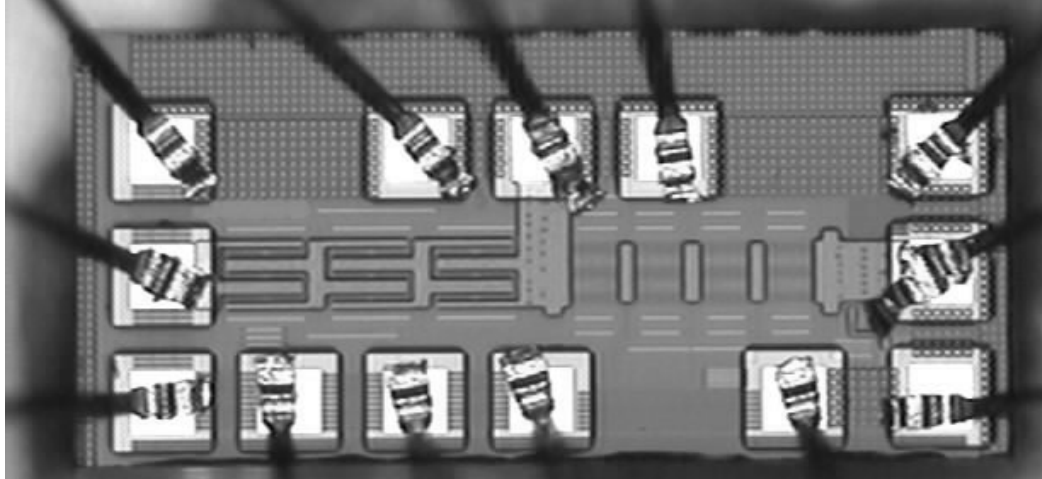
Fig. 4.38. Photograph of the CMOS switch using the Feed-forward capacitor
