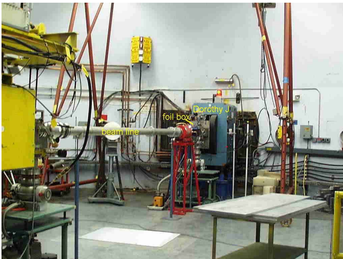
Figure 10: Blue room setup for foil irradiation at WNR. Protons enter from the left.
