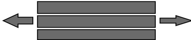
Figure 2.1 Voigt model: Uniform strain field in both phases
