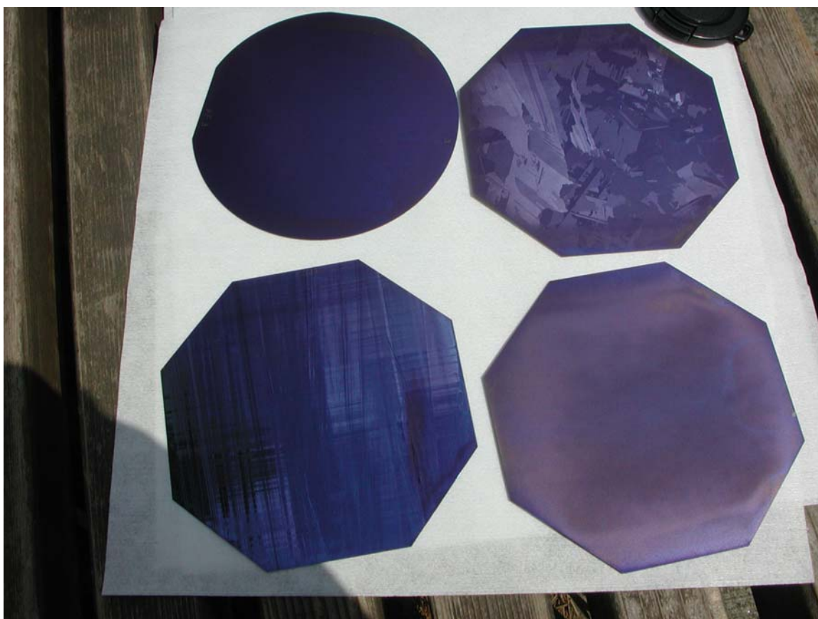
Figure 75. Porous silicon etched wafers after DOSS diffusion. Top left – FZ, Top Right – cast mc-Si, bottom left – EFG ribbon, bottom right – Cz.
