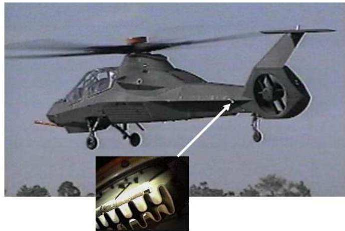
Figure 10: RAH-66 Comanche Mixer/Ejector Exhaust Infrared Suppressor System
