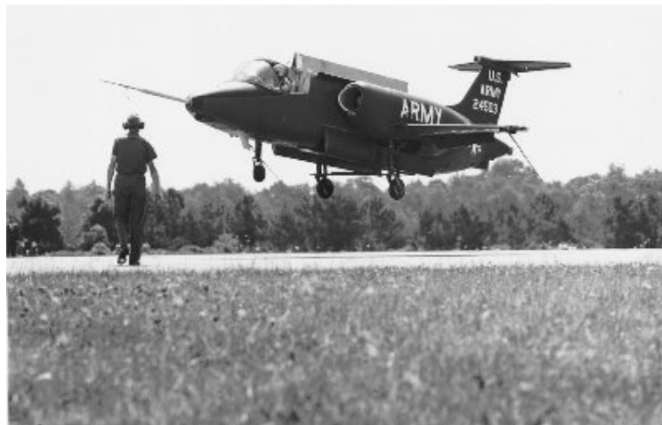
Figure 7: Lockheed XV-4A Hummingbird Hover Test
