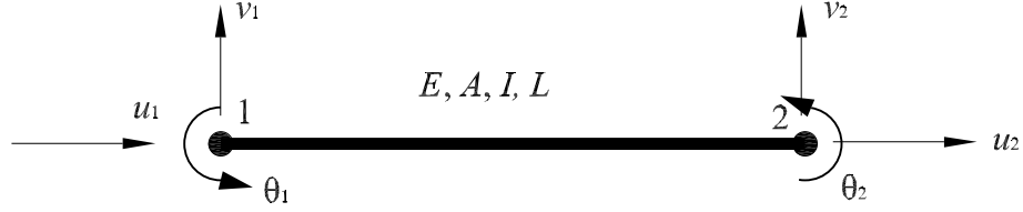
Figure 4.8: A frame element and its nodal d.o.f.
